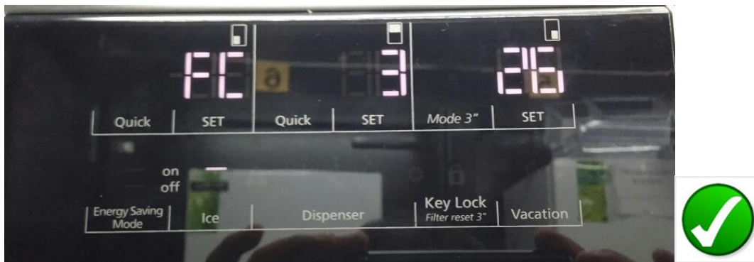
Figure 1. Software version and revision information on the display unit when the refrigerator is plugged in
